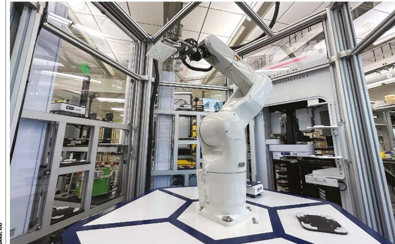
Leaps in technology are supporting AI-guided drug design, such as this fully robotic workstation that can purify proteins and move liquids.
