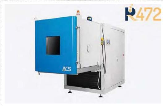
"Vibration test chamber"
